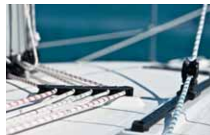
The genoa tracks are positioned on top of the coach roof, ensuring excellent up-wind characteristics. Short ways for the jib-sheets makes tacking easy
