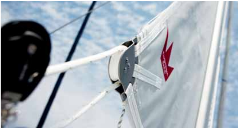
Roller furling mainsail and headsail ensure safe and easy handling for any size of boat
