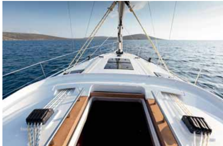
BAVARIA dual mainsheet, mid-boom sheeting system – enables exact trimming without traveller as well as safe gybing
