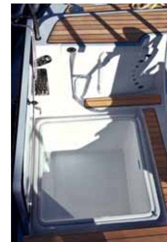
Larger cockpit locker for easy loading and unloading; additional storage under the cockpit floor
