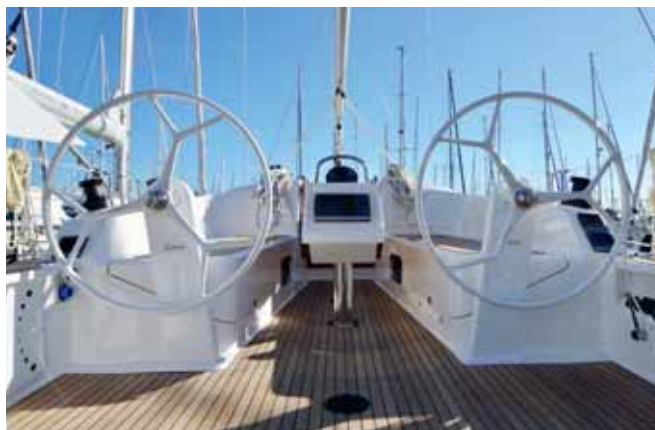
The twin-steering system of the CR 56, 51, 46, 41 und 37. Good cover through high spray hoods* and complete biminis* against wind and weather
