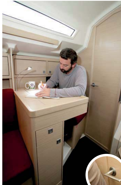
A good-size chart table but not much instrument space INSET The heads door handle is too close to my ribs
